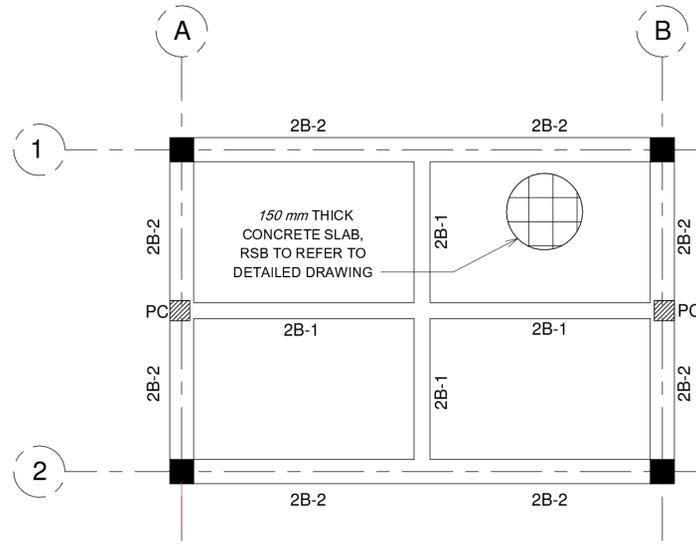
**5 ROOF FRAMING LAYOUT PLAN**
